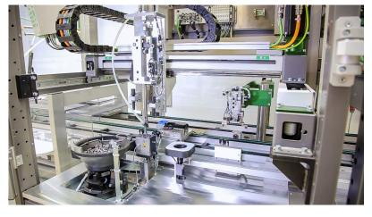
implementation of intelligent manual work stations without sacrificing processing reliability. The operator is taken step by step through the assembly task. Sensor technology activates the correct parameters for each screw position, releases fasteners, notifies the operator of subsequent tasks and evaluates results. The Pickand-Place procedure guides the operator by picking up the
