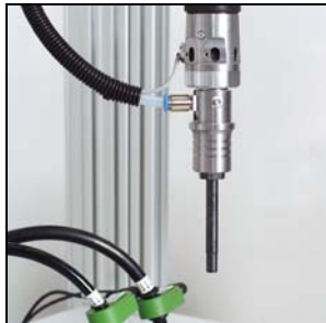
Particle Killer & vacuum tooling used for technical cleanliness
