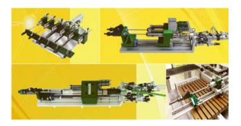
The screwdriving function module itself can also be equipped with optional added functions. The screw depth control, digital or analogue, checks the screwed assembly and ascertains whether the screw fastening has been carried out properly. This provides a high degree of process reliability for each step of production.
