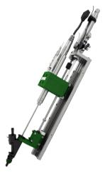
**short** version is particularly suited for operations where space is restricted. The **under-floor** version is designed for vertical screwdriving tasks from below. The **vacuum** version handles tasks in hard-to-reach or recessed screw locations in any direction. The **pick and place** version is used to deal with fasteners that have a specified pick position. The **nut feed** version feeds and screws nuts onto the fastenings.
