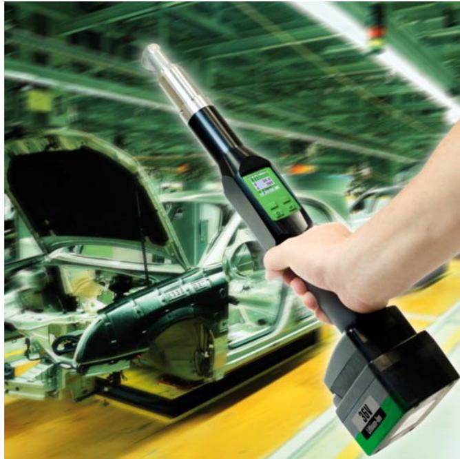
These new batteries have a considerably lower idle-discharge, and the dreaded memory-effect - that occurs as a result of partial charging - is non-existent. It is also important to note that the new batteries can now be fully charged in about 40 minutes.
