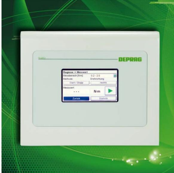
texts and symbols as well as color differentiation of the results (green or red) ease operation for the workers. The menu for the fc20's various features can be touch screen accessed. A clearly structured menu shows the way to the desired submenu, where the definition of sequences and programs or the selection of diagnostic functions is easily carried out.
