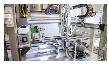
Fasteners are primarily fed to the screwdriving tool for processing via a feed hose from the feeding system. It is however, sometimes not possible to feed screws with a very short shaft, rivets with a large collar diameter or parts with particularly complex external geometry by feed hose. In this case the best option is the Pick-and-Place procedure in which the screws are "picked" using vacuum, gripper or magnet system. After
