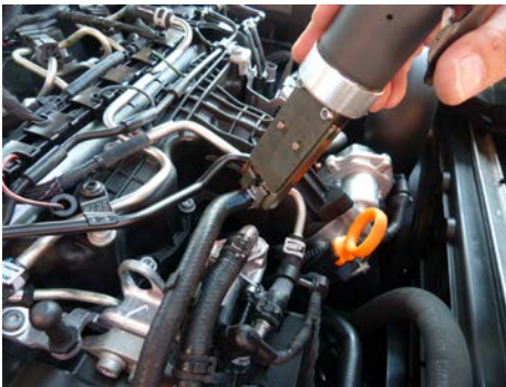
Application Example, Spring Clamps – Effortless installation of a cooling system tube clamp in a vehicle engine compartment
