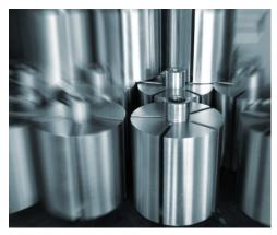
After enrichment with carbon, the steel rotor is hardened and then tempered (relaxed). During hardening the steel is heated to the austenite phase (over 723 degrees Celsius) and then quickly cooled (quenched) in order to circumvent the pearlite and ferrite phases and reach the so-called hardened martensite microstructure. The hardening procedure is followed by tempering (regulated reheating) process in order to give the steel back a certain degree of strength and ductility.
