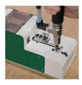
For the supply of screws with a shaft-diameter of 1 mm to 5 mm and a shaft-length up to max. 25 mm.
