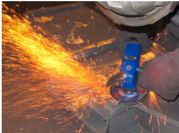
Grinder equipped with a cup wheel
