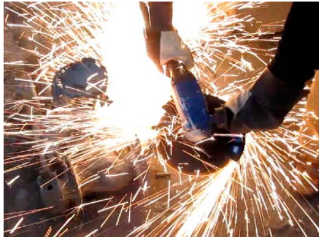
DEPRAG Turbine Grinder used in a Foundry
