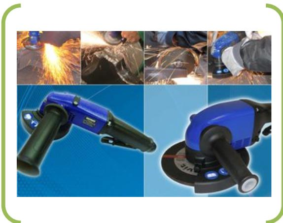
because maximum power is achieved only at half the no-load speed. Conversely, exceeding the speed of 80 m/s can result in disc rupture due to centrifugal force. In practice this problem has been solved by installing a speed regulator.
