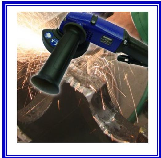
Particular attention has been paid to work safety. The safety valve on the right handle prevents the grinder from starting accidentally, and with its two-stage opening stroke, ensures low actuation forces; once released, it automatically reverts to the off position (“dead man’s switch”). An integral, redundant operation emergency-off switch stops the machine if the centrifugal force regulator fails, so that the worker and the environment are not at risk from rupturing grinding discs.
