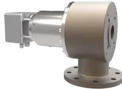
The innovative GET turbine generator converts the energy contained in the working fluid into power. Gas flows into the turbine, is "compressed" by jets, accelerated, comes into contact with the turbine wheel and releases energy. The kinetic energy is converted into electric energy in the generator. In this innovative system, the turbine and electric generator constitute a compact unit – they share a common shaft. Consequently: When the turbine turns, the rotor of the generator also turns.
