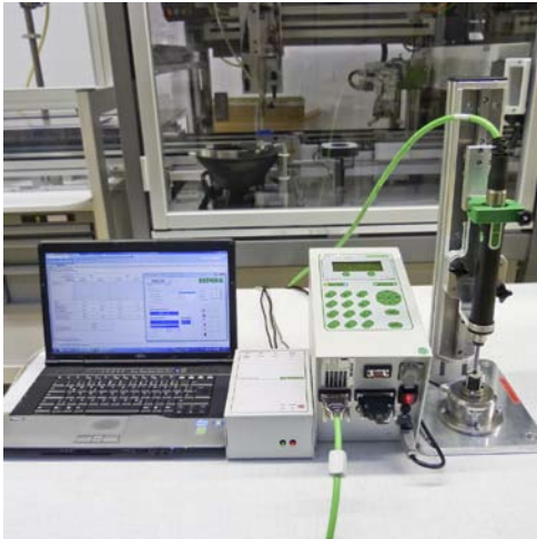
Calibration Setup - Screwdriver
