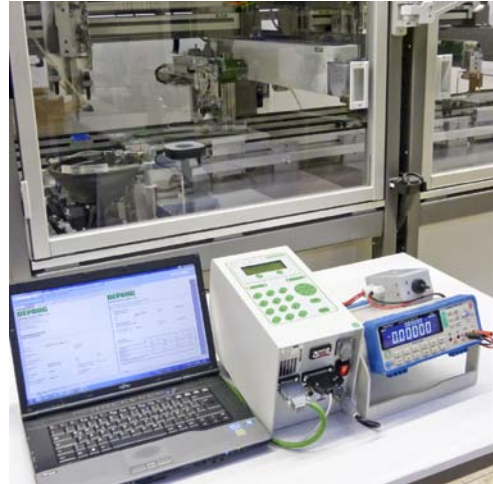
Calibration Setup - Controller
