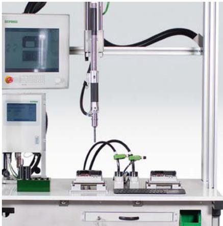
*Screwdriver with Controller and CleanFeed System*
