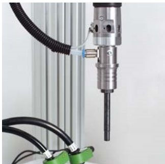
Vacuum Suction at the Screwdriver Tip
