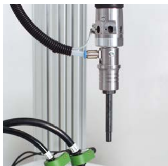
Vacuum Suction at the Screwdriver Tip
