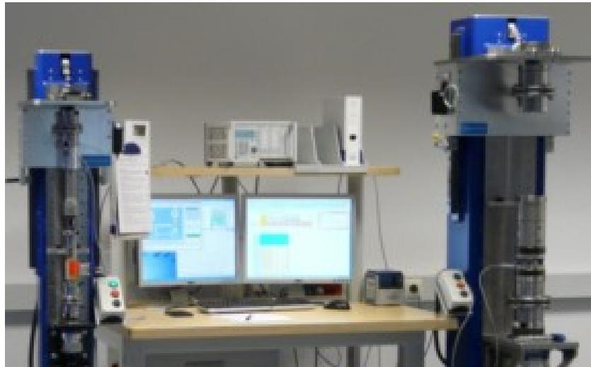
cases could be caused by an incorrect torque setting. It is then no surprise that the accuracy of assembly tools is a top priority for the automobile industry. Therefore modern assembly tools are equipped with torque transducers which are responsible for control, documentation, and recording of torque values during assembly.
