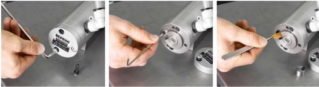
The DEPRAG patented Vane exchange feature on the Basic Line Motor
