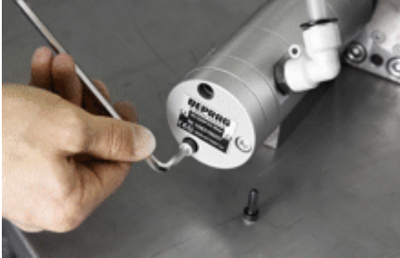
Detail of patented vane exchange feature http://www.depragusa.com/files/videos/lamellenwechsel.gif
