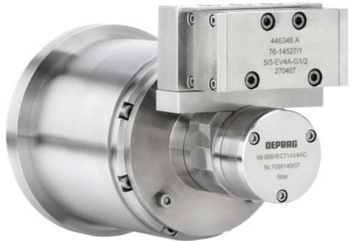
In addition, generated performance is almost constant over wide speed ranges. An air motor can also be operated over a wide load range. Motor performance can be modified by altering the operational pressure, while speed can be smoothly controlled by throttling the air quantity. An air motor can also be loaded to a standstill without causing any kind of damage. Once the load is reduced, the motor restarts immediately. This can be done as many times as required, even at high duty cycles.
