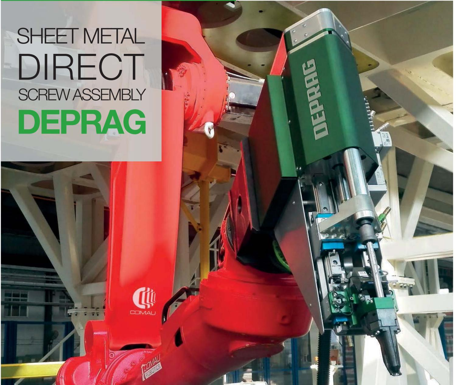
The **DEPRAG** FlowFormScrewdriving system for direct screw assembly of chassis components
